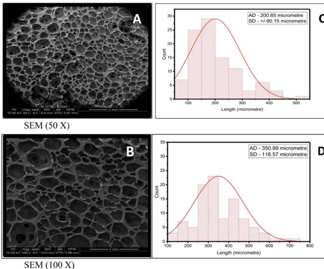
**Figure 1.** (A) SEM images of gelatin haemostatic sponge under 50 X magnification, (B) SEM images of gelatin haemostat under 100 X magnification, (C) pore size distribution of gelatin sponge under 50 X magnification, and (D) pore size distribution of gelatin sponge under 100 X magnification.
